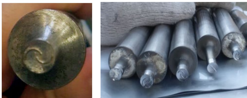
FIGURE 3 Tablet punches with the characteristic Captagon logo comprising two half-moons, found in dismantled illicit laboratories
